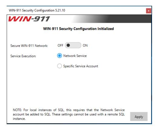
Flipping the switch to "ON" will secure the connections between the installed modules.
